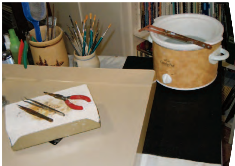
A complete solder station, with tweezers and “burn ‘em up” pliers.
