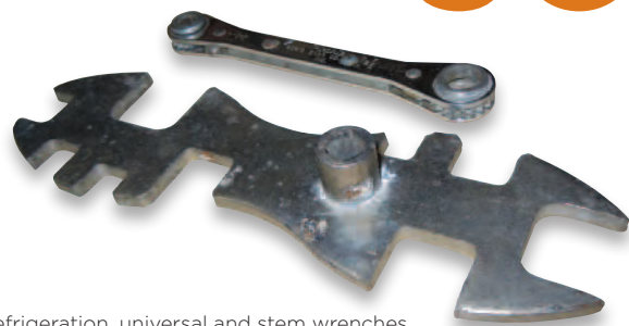
Refrigeration, universal and stem wrenches.
