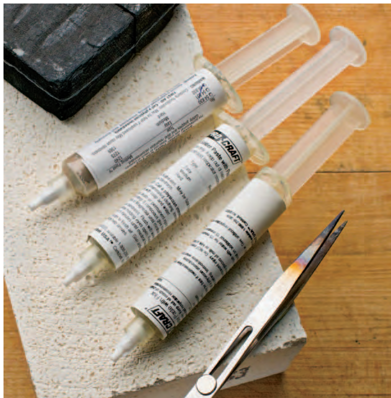
Paste solder is handy for workshops and classes because the flux is already mixed in. Photo: Jim Lawson
