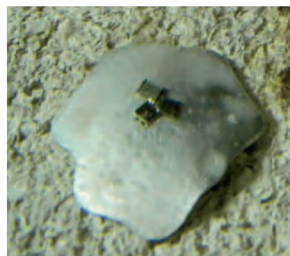
Fresh flux and solder pallions prepped for sweat soldering.
