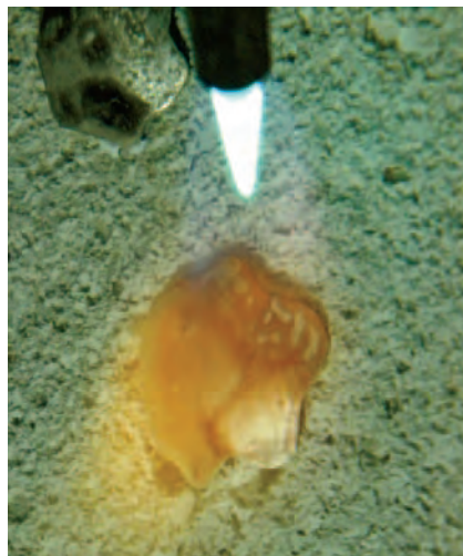
Danger zone! Don't get your piece too hot: you'll be in danger of a meltdown, and you'll destroy the protective properties of the flux.
